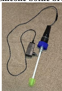
Figure 2. Closer view of Agitator made using silicone bottle brush
