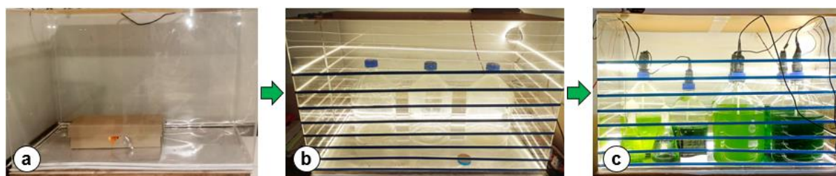
Figure 1. Steps involved in construction of a photobioreactor: a) Construction of a photobioreactor using acrylic sheet b) Fixing of LED lights on photobioreactor for illumination c) Algal cultures efficiently growing in bottles fixed with silicone bottle brush agitator system
